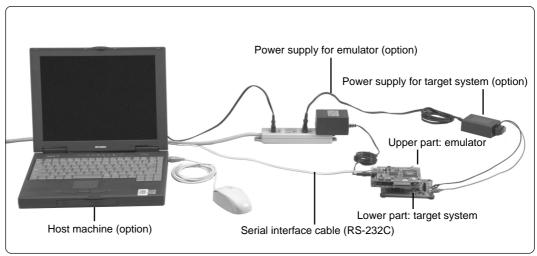
Figure 2.1 System configuration
